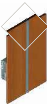
UNDERCUT CONCEALED FIXATION WITH JOINT CONNECTOR
